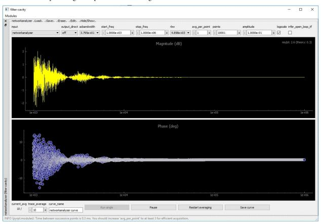
The network analyzer records the coherent response of the signal at the port input to a sinusoidal excitation of variable frequency sent to the output selected in output\_direct.
