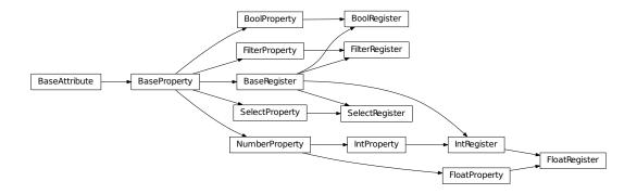
As for the distinction between software modules and hardware modules above, the properties that inherit from BaseRegister are directly mapping an FPGA register. On the other hand, software modules are using properties that are not in direct correspondance with an FPGA register. However, since they inherit from BaseAttribute, the load/save and GUI update mechanism is still implemented.
